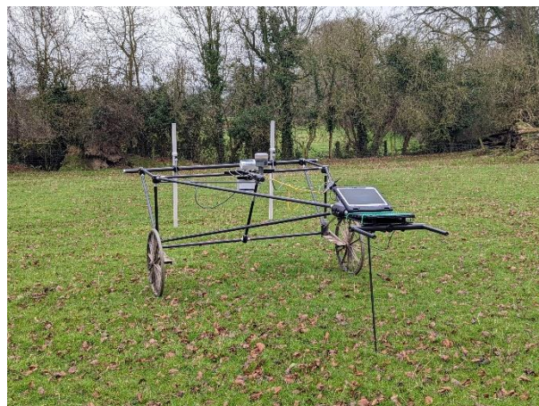
Bartington Grad 601-2 mounted on Bartington Cart
